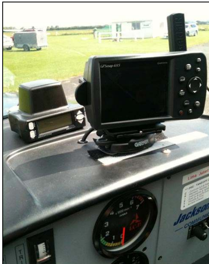
The Zaon unit mounted on the dash of LJW and the GPS sitting in the holder for it. The cables run around the back out of sight
